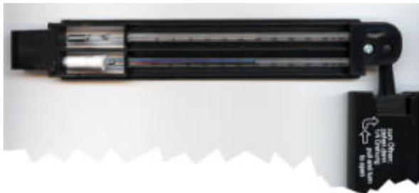
[6] Slide the instrument into the frame and use the scales on the back side to determine the relative humidity.
